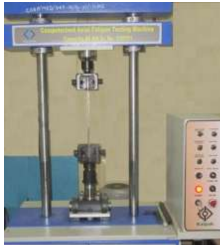
Fig. 2 Photograph of the experimental set-up for uni-axial fatigue testing.
